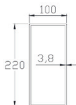
2 Column and Side Beam Profile
